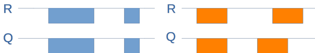
Figure 2.2: Example of anchor pairing: The blue anchors on the left are equidistant and form a pair, the orange anchors on the right are not equally spaced and are not considered. The anchors do not have to start at the same positions in the sequence.
