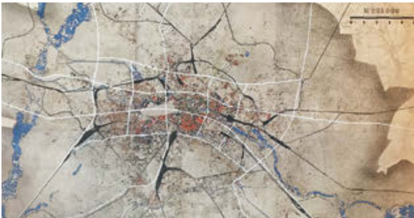
140, 141 Collective plan prepared by the planning collective, 1945/6. Original scale 1:10,000, 95 × 195 cm. The “green mist” that covered the entire central plan was meant to be a clear indicator of the complete “interpenetration” of built and green structure.
