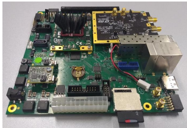
Figure 35 Carrier board “TEBF0808” equipped with the Trenz Module TE0803-04-4AE11-A and the FADC card “DC2266A” (with ADC Ltc2017). The heat sink covers the ZU+ device (on the Trenz Module). The front side of the also implemented RJ45 plug is not visible in this figure.
