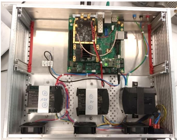
Figure 34 Equipped carrier board in final housing with its power supplies
