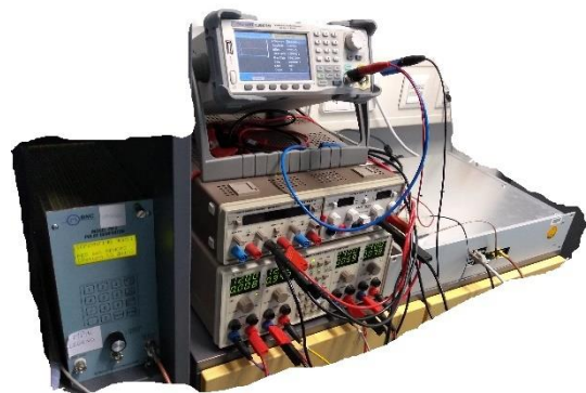
Figure 175 Several Regions PB-5 setup with FC2.0 prototype. The PB- 5 is visible on the left side of the figure. It needs an external (NIC compatible) power supply (at the bottom in the middle) to be operated. The SDG022X can be seen on the top of the power supplies.
