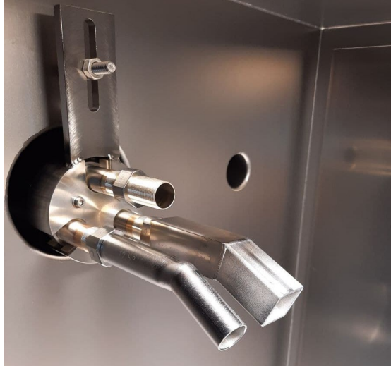
Figure 3.5. Photograph of the shatter heads in the shattering test chamber. At the topmost barrel, no shatter tube is mounted. 12.5^\circ mitre-bend shatter tubes with a circular (left) and rectangular (right) cross-section are screwed onto the bottom left/right barrels.
