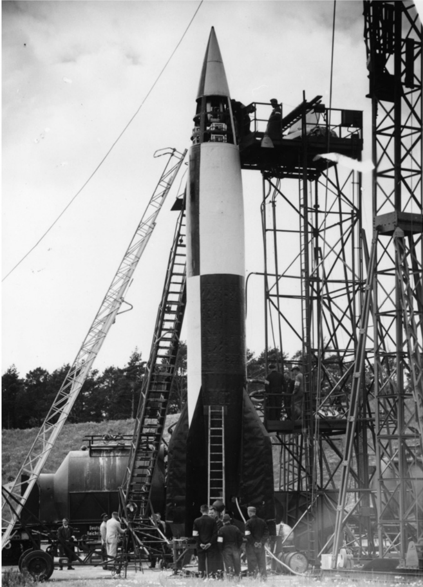
ILLUSTRATION 70 Preparation for the launch of an A-4 rocket, 1942: the control section of the world's first large rocket to travel in space, which was 14 meters high and weighed 12.9 tons with full tanks, is open; above there is space for a payload of one ton. The A4 missile (A stands for Aggregate), a series of ballistic rockets developed by Wernher von Braun's group in Peenemünde, was later named the V2, Vergeltungswaffe (weapon of retaliation).
