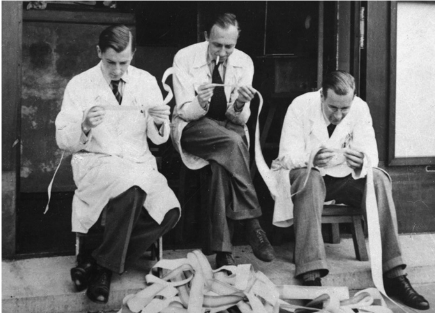
ILLUSTRATION 45 Wolfgang Gentner with Peter H. Jensen (on his right) and Arnold Flammersteld (left) during WWI, evaluating measurements of the energy of fission neutrons, whose pulses were recorded on photographic paper strips via oscillographs. The institute's Van de Graaff provided neutrons through the bombardment of beryllium with accelerated nuclei of deuterium.
