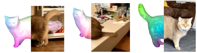
Figure 11: BANMo [YVN*22] uses a NeRF-style object representation to reconstruct an object from a few monocular videos. Image adapted from [YVN*22].
