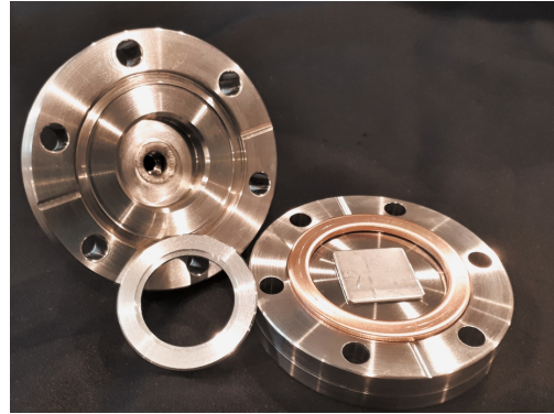
Figure 5: Emanation vessel used for the measurement of the sample's radon emanation rates. The aluminum ring (front) is used to fix the sample in place.
