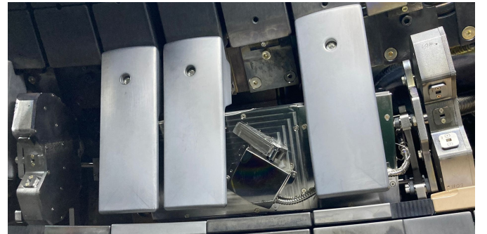
Fig. 11. INPA head being protected from the radial heat flux by three graphite protections.
