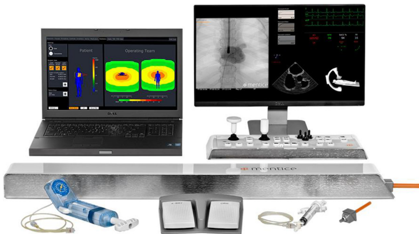
Fig. 2. Endovascular simulator VIST G5 (Mentice, Gothenburg, Sweden) including the fluoroscopy screen, human body dummy, syringe to inject contrast agent, control panel to move the patient table and foot paddle to control the x-ray usage (Image courtesy of Mentice - Mentice VIST® G5 simulator - 16.11.2022 - www.mentice.com).
