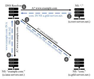
Figure 8: Simplified overview of DNS resolution for IN A www.example.com.: (1) The resolver asks the root-servers for www.example.com., (2) The resolver is redirected to the authoritative NS for com., (3) The resolver asks the com. NS for www.example.com., (4) The resolver is redirected to the authoritative NS for example.com., (5) The resolver asks the example.com. NS for www.example.com., (6) The resolver receives the A RRset for www.example.com. in response.
