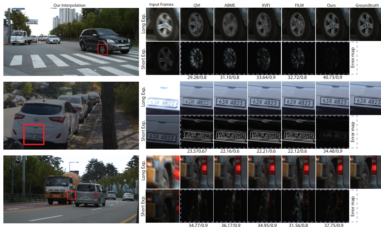
Figure 5: Visual comparisons of our method with the state-of-the-art VFI methods using the synthetic dataset described in Sec. 6.1. For each of three scenes, the first row of insets shows the performance of respective VFI methods, while the second row presents the corresponding per-pixel error maps between the interpolated results and the ground truth. The PSNR/SSIM values written below each error map are computed for each inset rather than the entire image. In the upper scene taken from the X4K1000FPS test set, the wheel moves in a non-linear trajectory and the existing VFI methods struggle to position the wheel correctly for the interpolated frames, while our method leads to a good alignment with the ground truth. In the middle scene taken from the GoPro dataset the camera is moving with an extremely non-uniform motion as shown in Fig. 3. While the existing VFI methods produce visually plausible results, they are not correctly aligned with the ground truth as the error map reveals. The bottom scene, taken again from the X4K1000FPS test set, contains a combination of camera and object movements. In this case, the existing VFI methods fail to properly handle the occlusion boundaries.
