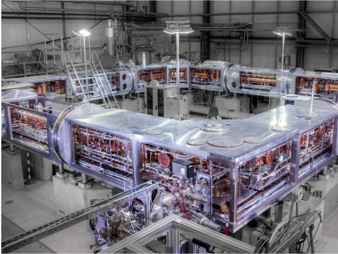
Figure 1.6: Photograph of the Cryogenic Storage Ring (CSR). For demonstration purposes the outer walls of the vacuum chambers have not been mounted yet. (Credits: Christian Föhr 2013)
