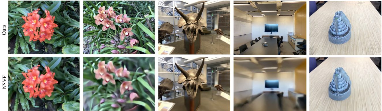
Figure 3. Comparison to NSVF [16] in Novel view synthesis. As discussed, NSVF struggles with real frontal scenes, in which the content is not captured from 360^\circ .
