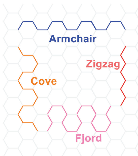
Scheme 3. Representative edge structures of GNRs.
