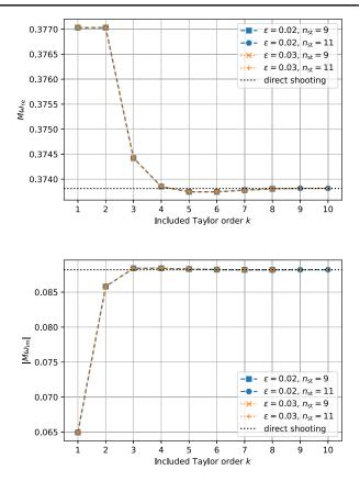
FIG. 7. Here we show the real part (left panel) and imaginary part (right panel) for the n = 0 quasinormal mode computed for the mixed potential for different step-sizes  $\epsilon = (0.05, 0.1)$  and stencils of  $n_{\rm st} = (9, 11)$ . The direct shooting values are indicated as black dotted line.
