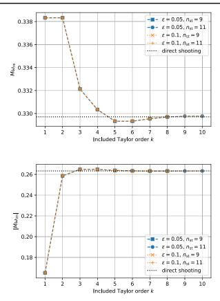
FIG. 6. Here we show the real part (left panel) and imaginary part (right panel) for the n = 1 quasinormal mode computed for the BW potential for different step-sizes  $\epsilon = (0.05, 0.1)$  and stencils of  $n_{\rm st} = (9, 11)$ . The direct shooting values are indicated as black dotted line.
