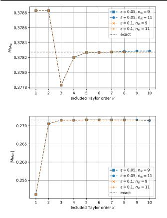
FIG. 4. Here we show the real part (left panel) and imaginary part (right panel) for the n = 1 quasinormal mode computed for the PT potential for different step-sizes  $\epsilon = (0.05, 0.1)$  and stencils of  $n_{\rm st} = (9, 11)$ . The analytic values are indicated as black dotted line.
