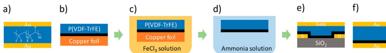
Figure 3.1. a) P(VDF-TrFE) capacitor and the chemical structure of P(VDF-TrFE). b) to f) Schematic description of the fabrication process of the graphene Fe-FETs and MIS-diodes. b) P(VDF-TrFE) is coated on top of the CVD-grown graphene on Cu foils followed by Cu etching in c) and ammonia washing, d). The graphene layer is subsequently transferred using a conformal transfer onto a pre-patterned FET substrate e) or an Au-coated glass substrate for the MIS-diode f). The P(VDF-TrFE) layer serves as both the transfer layer and the gate dielectric.
