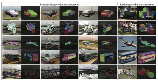
Figure 2. An overview of our UDA-Part dataset. UDA-Part is a comprehensive part segmentation dataset for five vehicle categories. Each category is composed of several 3D CAD models/prototypes. By labeling parts on these 3D CAD models, we render a large-scale synthetic image dataset with automatically generated part segmentation ground-truth (left panel). To benchmark unsupervised domain adaptation methods, we also label parts on a moderate number of real images for testing (right panel).
