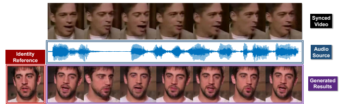
Fig. 6. Illustration of the audio-driven talking face generation task. With one frame as the identity reference, the task aims to synthesize talking faces that are aligned with the given audio source. The image is adapted from [53].
