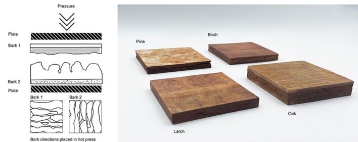
Fig 2. Arrangement of the bark pieces in the hot press (left). Produced panels with in-plane dimensions of 10 x 10 cm 2 and variable thicknesses determined by the natural structure of the pressed bark pieces (right).
