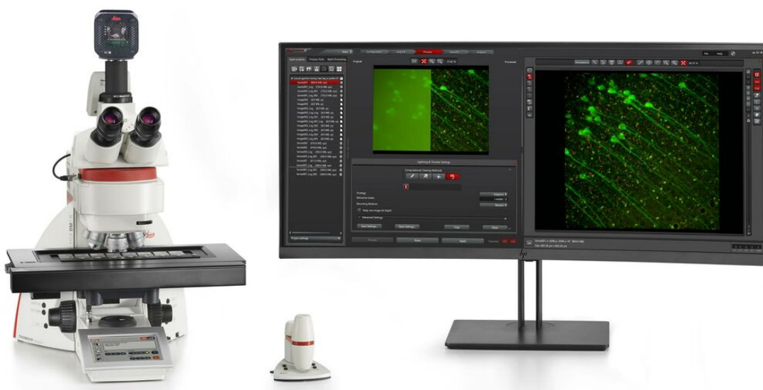
Figure 34: Leica Thunder microscope coupled to a Leica DFC9000GTC-VSC12365 camera [95]
