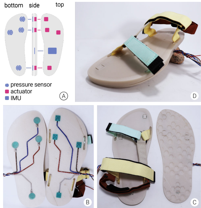
Figure 4: The first iteration of the augmented footwear: (A) Positioning of the sensors and actuators; (B) The bottom and top part of a sandal with four FSR sensors (left) and four actuators (right) embedded into the sole with silicone inlays; (C) The top part with off-the-shelf straps (left) and the profile of the bottom part (right); (D) The fully assembled sandal.
