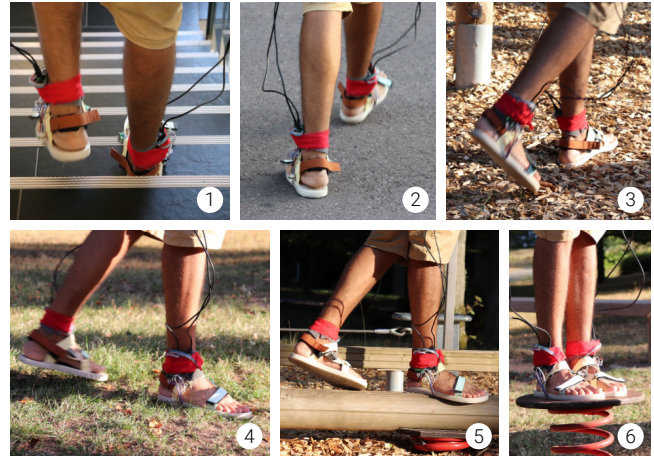
Figure 7: In preliminary tests, the authors explored the experience of walking with the augmented sandals on different surfaces, i.e. (1) walking up and down stairs (stone), (2) asphalt, (3) wood chips, (4) grass, (5) tree trunk, and (6) balancing on a springy plate.
