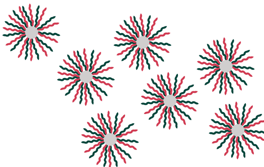
Figure 4-1: Amphiphilic binary mixed brushes for stabilization of nanoparticle dispersions in media with various polarities.
