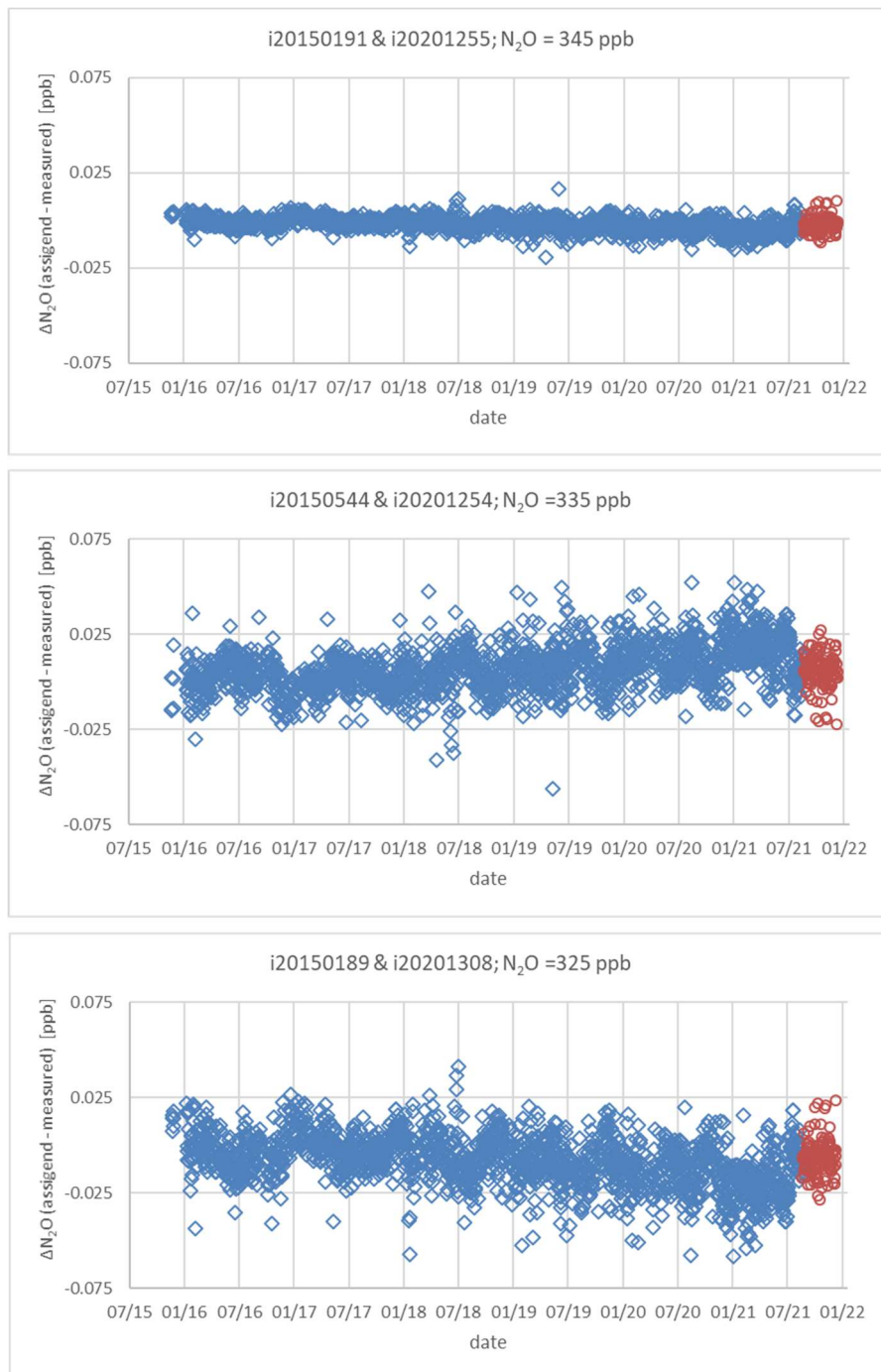
Figure 34: Quadratic regression fit residuals of the daily LGR N 2 O calibration with FCL Secondary Standards
