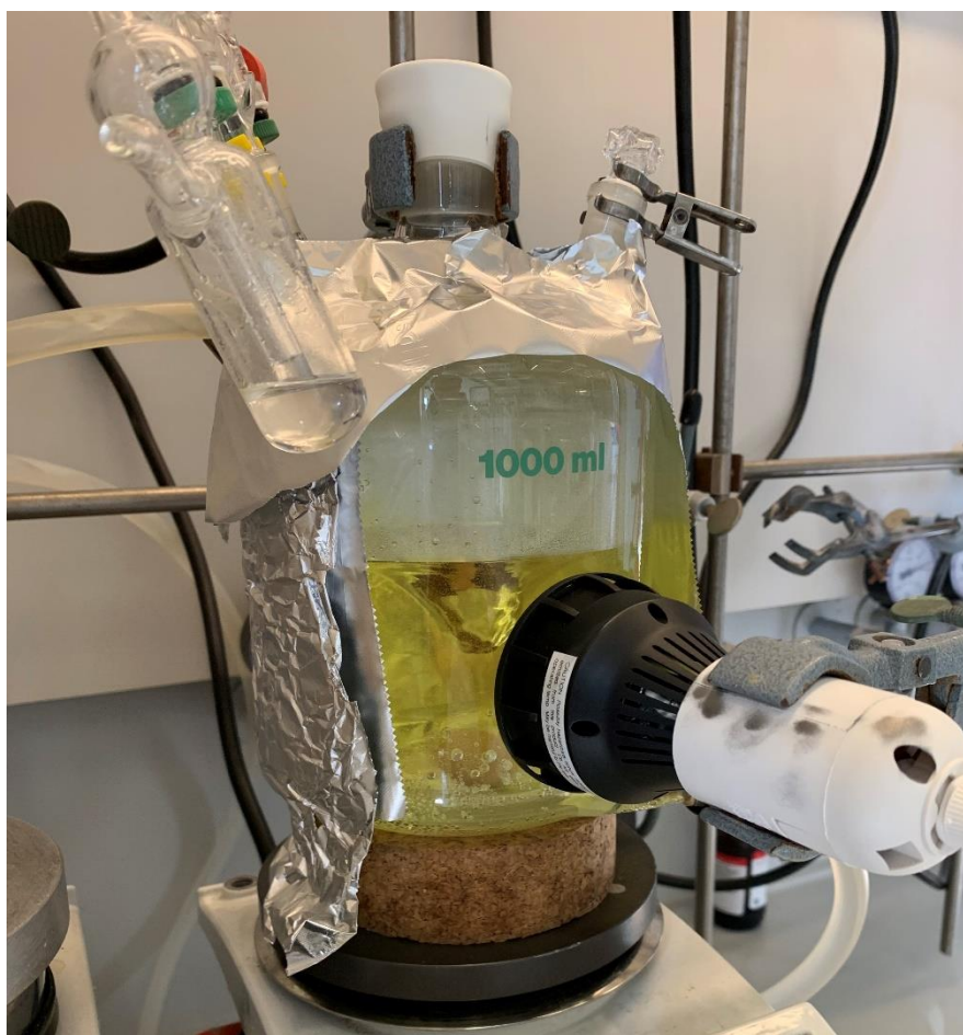
Figure S2. Reaction setup for the photosensitized [2+2] cycloaddition
