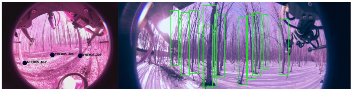
Fig. 7 Automated bounding box extraction (right) for the fisheye rgb camera data object detection using the extrinsic calibration (left) which can be combined with the meta information like diameter or specie.
