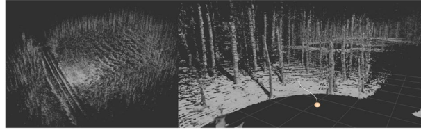
Fig. 13 Qualitative results of TSDF based map generation using Voxblox 31 . The figure shows the result of (h1f1r1). The left a global view and the right zoomed near-field. Trees and paves are clearly visible. The representation can be directly used for path planning.
