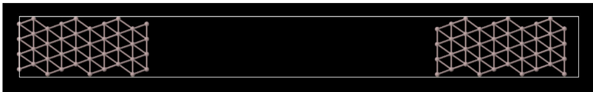
Figure C.4: Typical dimensions of a 2-electrode setup in SMEAGOL or TranSIESTA with 6 atomic layers in a principal layer.
