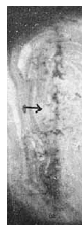
Figure 14. Image of the deflection pattern for iron atoms in an inhomogeneous magnetic field of 200 kG/cm. No deflected Fe atoms were detected. The arrow marks the maximum inhomogeneity of the magnetic field. See also text and Table 1. Reproduced from Ref. [25].
