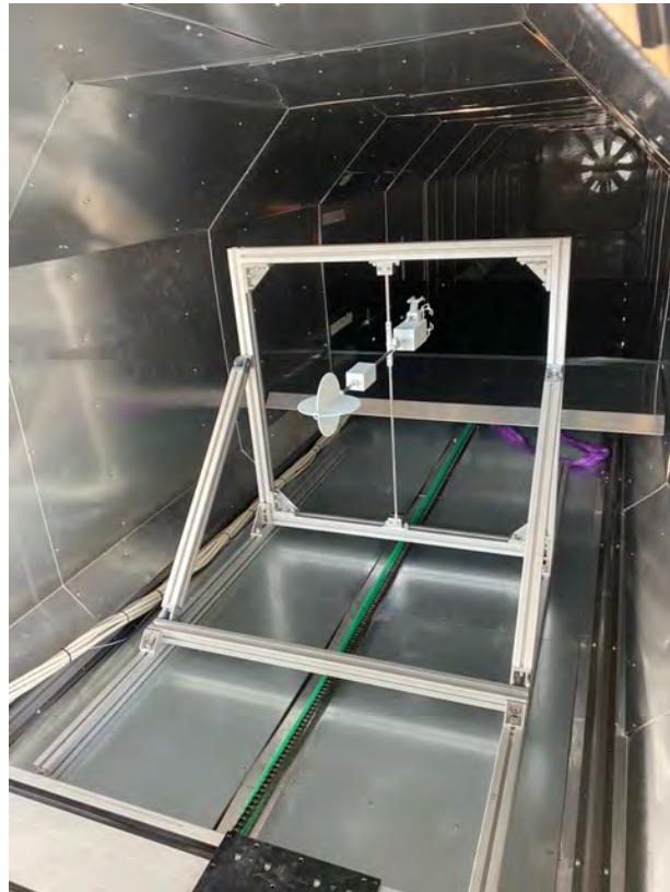
Figure 2.18 The 1:4 mini-MPCK model is mounted to a frame of aluminum profiles inside the Prandtl tunnel. In the background, the fan is visible. The mini-MPCK is close to the outlet and points to the mean wind direction.
