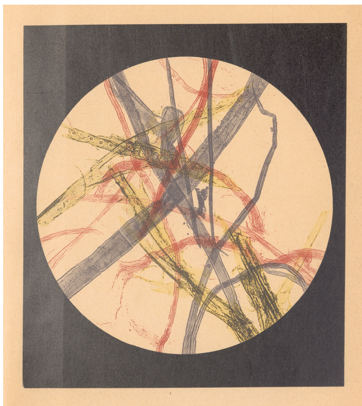
Figure 2. Microscopic representation of the dyeing of linen and cotton, wood and straw pulp, and wood pulp fibers in chlor-zinc-iodine solution. From Wilhelm Herzberg, Papier-Prüfung (Berlin: Springer, 1894), Plate 14.
