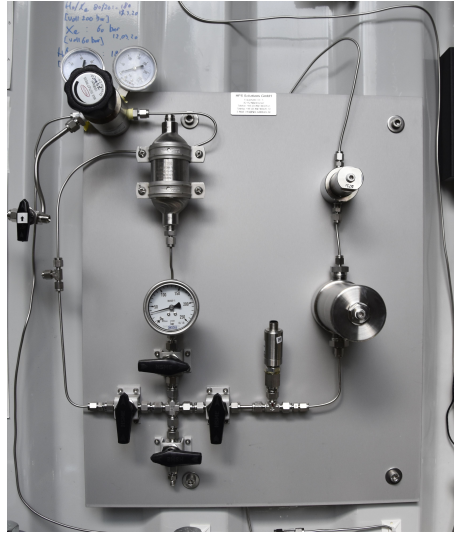
Figure 3.10: Control panel of the HPS. Gas enters from the CS at a pressure of 10 to 200 bar, passes two filters and is stored in a 75 \text{ cm}^3 tank. The pressure outlet leading to the nozzle is controlled manually via a pressure reducer.
