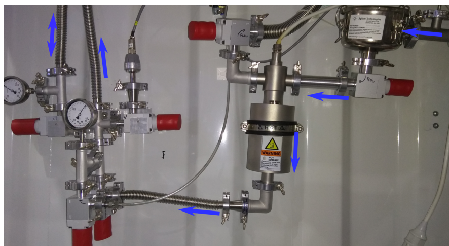
Figure 3.8: Setup of the LPS. Gas enters either via the exhaust of the SP set behind the turbo pumps through the filters, or comes directly from an external gas bottle. It is then stored in a 20 L tank and directed to the CS. The flow direction of target gas during recycling is indicated by the blue arrows.
