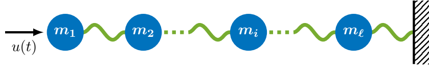
Figure 1: Schematic illustration of the Toda lattice with \ell particles [35]. Atoms in a one-dimensional crystal structure are represented as point masses and connected by exponential springs modeling the forces between the particles.
