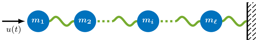
Fig. 4 Schematic illustration of the Toda lattice with \ell particles [39]. Atoms in a one-dimensional crystal structure are represented as point masses and connected by exponential springs modeling the forces between the particles
