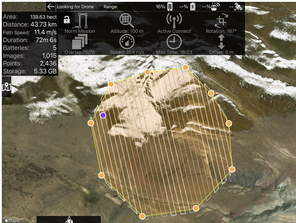
Figure 8. UAV flight plan in Map Pilot Pro from the MAPSS survey in Khovd.
