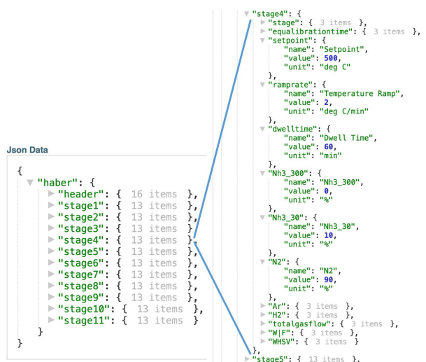
Figure 8. Metadata is not entered into predefined fields, but is contained in a single field in the form of JSON scripts, which can also be searched. These scripts are both machine- and human-readable. Here, metadata of an automated test reactor is shown and exemplarily unfolded, revealing the setpoint temperature and the heating rate in test segment 4 of an experiment and what gas composition is used. [90]
