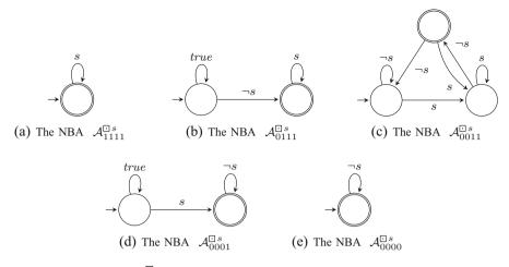
**Fig. 1** The Büchi automata  $\mathcal{A}_{\mathcal{B}}^{\boxdot s}$  constructed in Step 1 of our monitor construction
