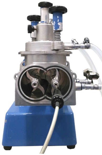
FIG. 3. Measuring kneader used for agitation and measuring torque. Showing open trough with inserted thermometer.
