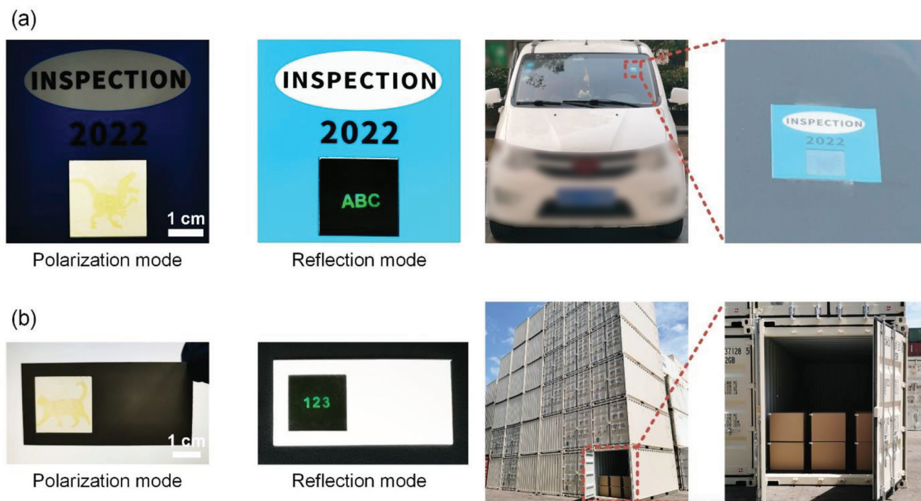
Figure 7. a) An inspection certificate for a car using anti-counterfeiting patterns of MC-Azo. b) Anti-counterfeiting labels of MC-Azo for products transported by containerization. Each package was labeled with an anti-counterfeiting label.
