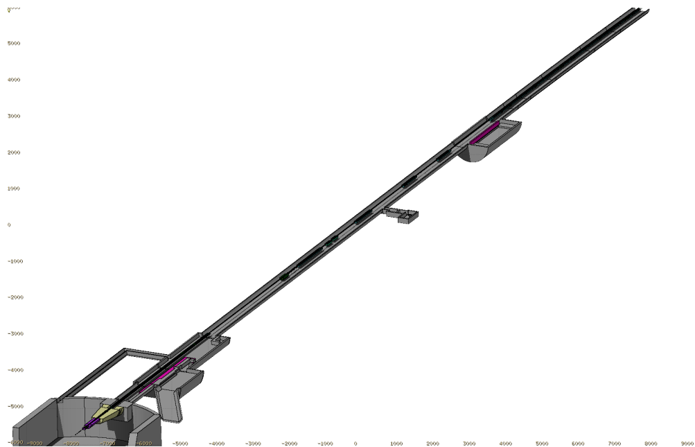
Figure 2.20: View of a portion of the FLUKA model of the HL-LHC. On the bottom left, one can see the ATLAS forward shielding surrounding the TAXS. The LHC tunnel extends to the west of the ATLAS IP up to the first DS cells (top right), with the violet wall shielding the RR alcove that sits at 250 m from the ATLAS IP.
