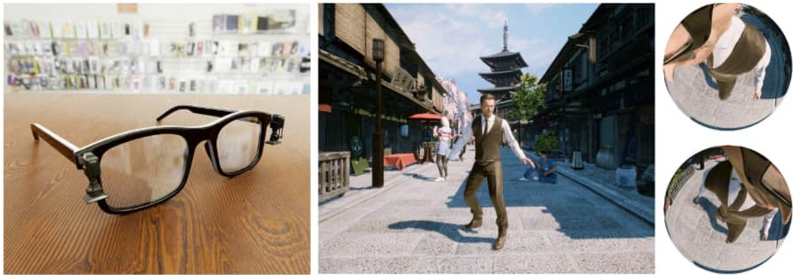
Figure 32.2: Egocentric pose estimation: proposed concept of glasses equipped with two fisheye cameras (a), a virtual human model wearing the glasses (b), and the rendered egocentric views (c).
