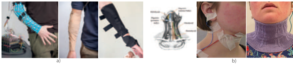
Figure 30.22: Left three panels show Skillsleeves which sense human actions and can actuate humans [2]. Right three panels show Vocal EMS for direct vocal control over vocal augmentation [7].
