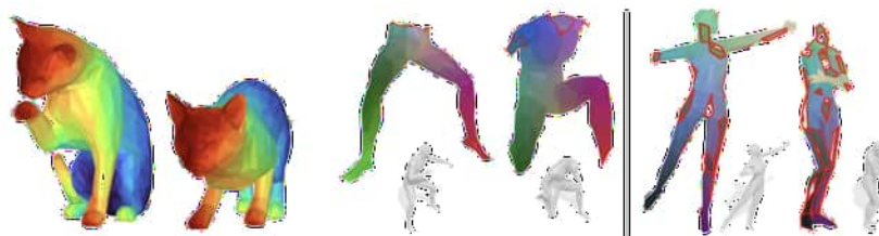
Figure 28.78: Orientation preserving shape matchings on triangle meshed. Matchings between complete shapes (left) and also matches between partial shapes (partial-to-partial shape matching) can be computed. Colors indicate matched triangles.
