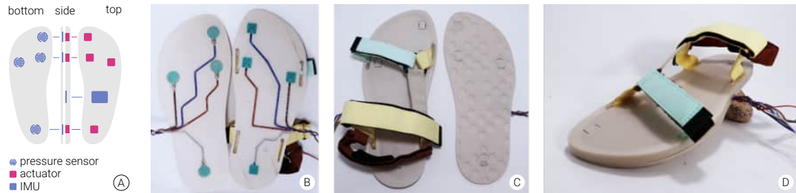
Figure 30.26: The Haptic Shoe consists of four pairs of pressure sensors and vibrotactile actuators and an IMU. The electronics are integrated in two-part 3D printed insole which forms the basis of a sandal.
