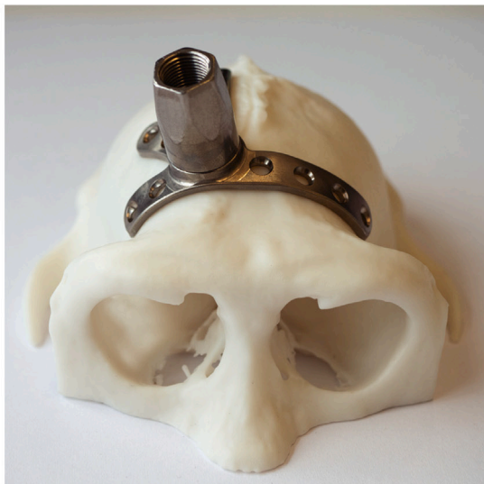
Fig. 2. The modular headpost implant. A) The main parts of the headpost are shown: on the left, a baseplate (flat precursor of bent version shown as example) with the cover screw, and on the right, a top part and the titanium screw that secures the two parts together (top-part screw). B) The CNC-milled version of the baseplate (frontal version) is shown on top of the 3D printed skull replica of Monkey H. C) The top part is added on the baseplate.
