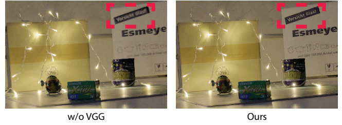
Fig. 13. Comparisons of the reconstructed HDR without and with the VGG loss (Ours). Our method synthesizes sharper details.
