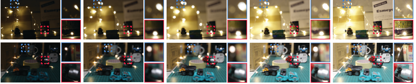
Fig. 4. Novel views with varying exposure time, aperture and focus distance synthesized by our method.
