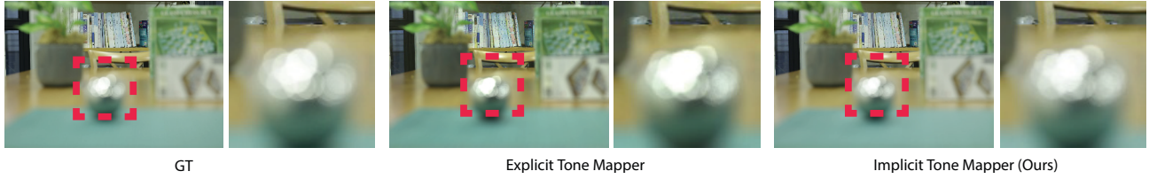
Fig. 7. Comparing LDR outputs of an explicit tone mapper to our implicit approach. The explicit solution struggles with the accurate reproduction of out-of-focus highlights.
