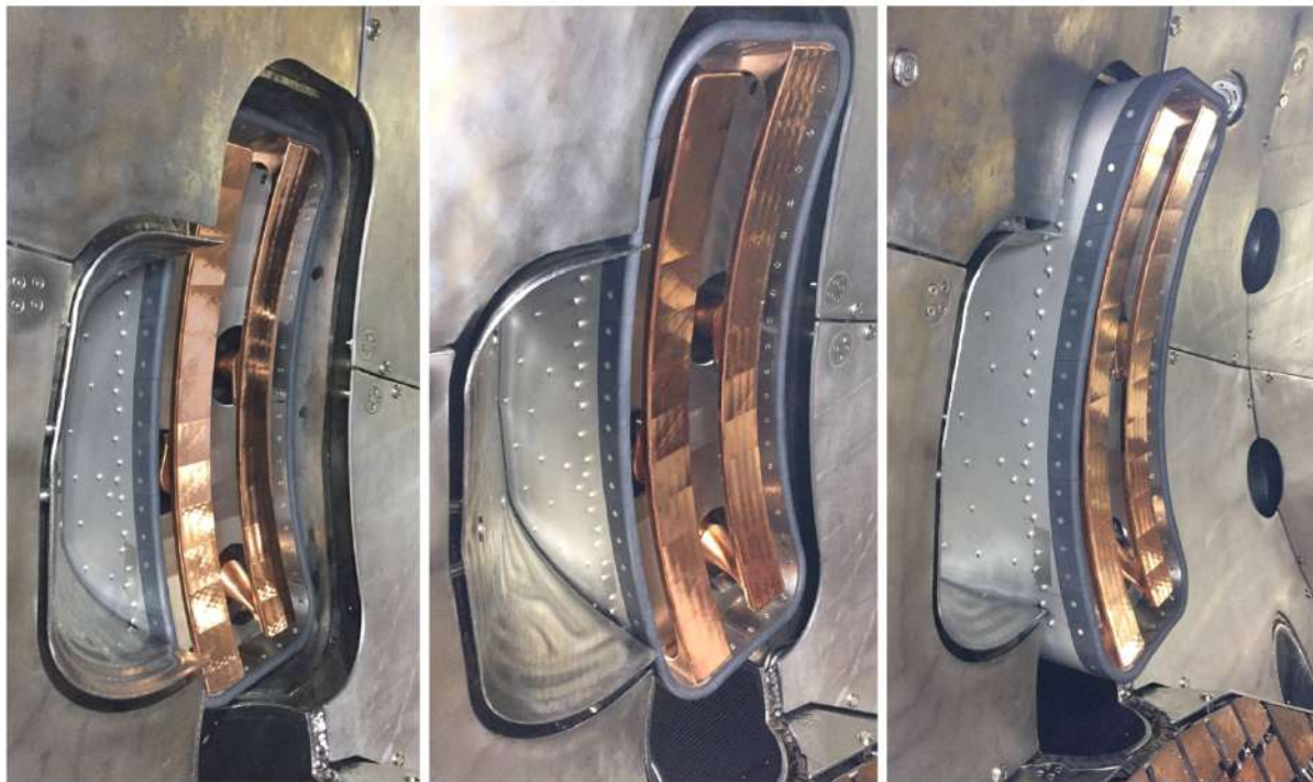
FIGURE 3. The radially moveable ICRH antenna in three different positions inside W7-X.
