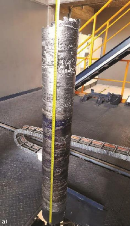
Figure. Illustrations of the successive steps of this work. A) PAM-CHR ingot, b) powder particles, c) large SPS billet, d) microstructure of the IRIS alloy and e) comparison of the creep properties at 800°C-200 MPa of the IRIS and IRIS+ alloy
