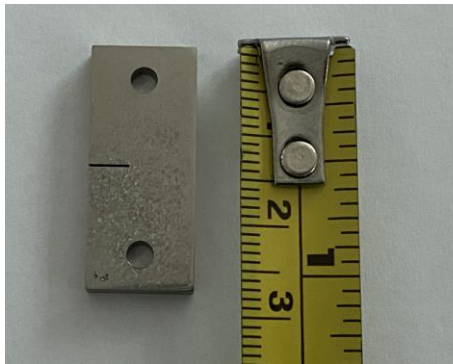
Fig. 1: Sub-size SENT specimen employed for the fatigue crack growth tests
