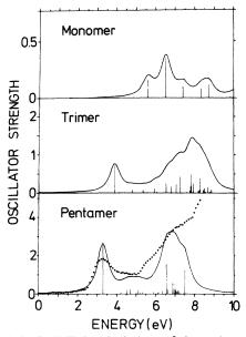
FIG. 8. LCAO-CNDO calculations of the  $\pi$ -electron oscillator strength of the monomer, trimer, and pentamer of pyrrole (solid curve). Points give the oscillator strength  $\omega \epsilon_2$  measured on the chemically reduced sample PPY-OS in arbitrary units.
