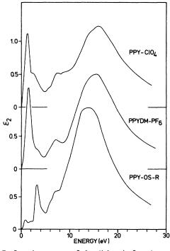
FIG. 7. Imaginary part of the dielectric function,  $\epsilon_2$ , as derived from a Kramers-Kronig analysis of the loss function of PPY-ClO<sub>4</sub>, PPYDM-PF<sub>6</sub>, and PPY-OS-R (electrochemically reduced).
