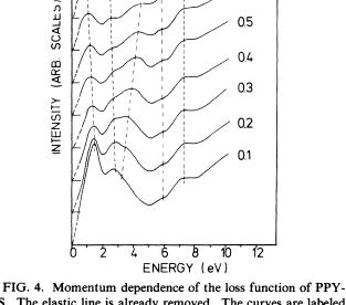
BS. The elastic line is already removed. The curves are labeled according to the momentum transfer.
