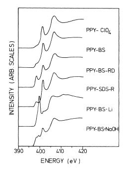
FIG. 10. Nitrogen 1s core-level excitation spectra in the energy range 390-420 eV for various pyrrole-based polymers. The curves are labeled with abbreviations explained in Table I. The label RD denotes after prolonged radiation damage in the electron beam. The labels R, Li, and NaOH denote electrochemically reduced samples, samples chemically reduced with Li, and NaOH-treated samples, respectively.
