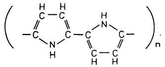
The structure of PPY films is reviewed by Street *et al.*<sup>5</sup> Electron-diffraction patterns<sup>6</sup> and x-ray diffraction<sup>7</sup> indicate a kind of layered structure with poor crystalline order. Compared to other conducting polymers like *trans*-PA or polyparaphenylene (PPP) the structure of PPY films is still rather unknown.
