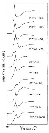
FIG. 9. Carbon 1s core-level excitation spectra in the energy range 200-300 eV for various pyrrole-based polymers. The curves are labeled with abbreviations explained in Table I. The labels *R*, Li, and NaOH denote electrochemically reduced samples, samples chemically reduced with Li, and NaOH-treated samples, respectively.
