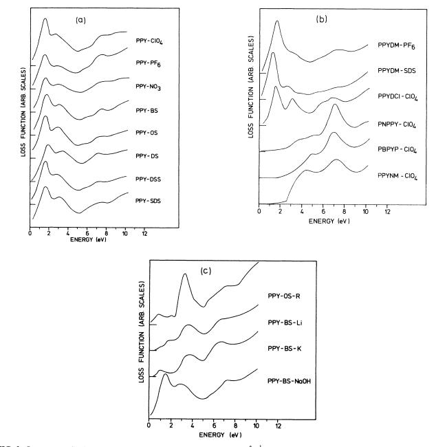
FIG. 3. Loss spectra in the energy range 0-10 eV, measured for  $q=0.1 \text{ Å}^{-1}$ . The elastic line is already removed. (a) as-grown oxidized nonsubstituted samples. (b) as-grown substituted samples. (c) Electrochemically reduced sample PPY-OS-R and chemically reduced samples PPY-BS-Li and PPY-BS-K, as well as NaOH-treated sample PPY-BS-NaOH.
