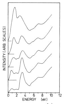
FIG. 6. Loss function, taken at q=0.1 Å<sup>-1</sup>, for PPY-OS for various reduction rates. Uppermost curve: oxidized sample asgrown. Lower curves: after increasing electrochemical reduction. Lowest curve: almost neutral PPY.
