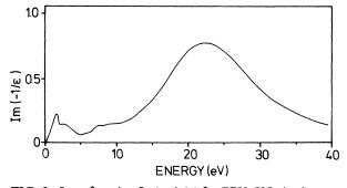
FIG. 2. Loss function  $Im(-1/\epsilon)$  for PPY-ClO<sub>4</sub> in the energy range 0-40 eV, measured for q=0.1 Å<sup>-1</sup>. The elastic line as well as contributions from double scattering are already removed.
