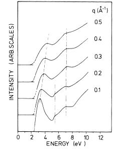
FIG. 5. Momentum dependence of the loss function of electrochemically reduced sample PPY-OS-R. The low-energy transitions are removed for clarity.
