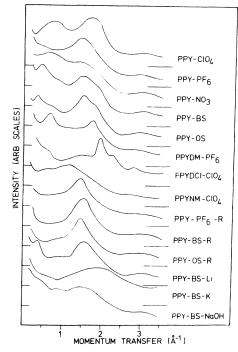
FIG. 1. Electron-diffraction patterns of pyrrole-based films. The curves are labeled according to their counterions and substituents as explained in Table I. The label PPY-BS-R denotes polypyrrole with butanesulfonate anions, electrochemically reduced. The labels Li, K, and NaOH denote treated samples as described in the experimental section.
