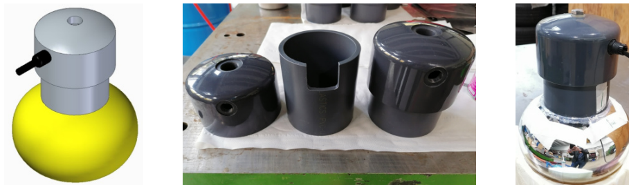
Figure 42 Left: Drawing of a Hamamatsu R5912 with encapsulation. Middle: Parts for the PMT encapsulation made of PVC-U. Right: Photo of a potted R5912 with encapsulation and cable.
