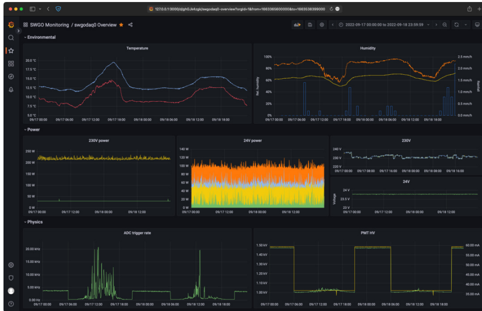
Figure 56 The visualisation of field node related data in one window. The dashboard includes in the top row environmental data, in the middle row measurements of the supplied power and in the bottom row physics data like trigger rates from the FlashCam readout and PMT voltages from the PhantomHV system.
