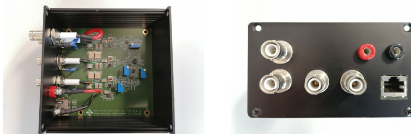
Figure 18 Left: Assembled Opamp Test Board with three different opamps. Right: Front panel with SHV connectors for PMT and for HV supply. RJ45 socket for output of the shaped signals to the ADC. Banana sockets in red and black for connecting 24 V board operating voltage.
