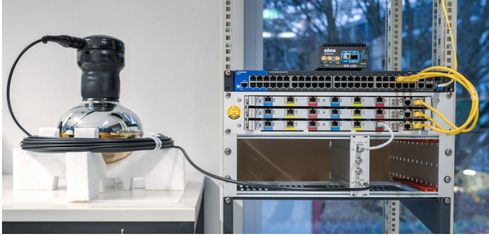
Figure 12 Measurement chain with a Hamamatsu PMT R5912-100, a PhantomHV System, a 24-channel 250 \text{ MS}^{-1} 12-bit ADC (FlashCam), a standard 10 GbE network switch, and a commercial White Rabbit slave for sub-nanosecond clock synchronisation.
