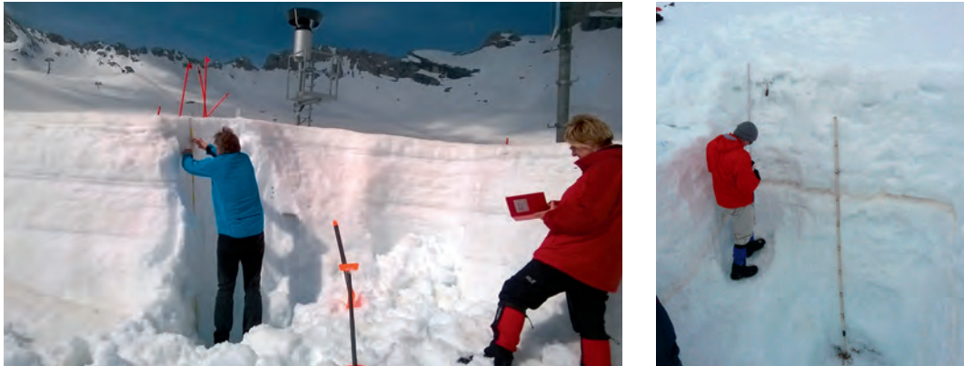
Fig. 3: Snow profile description and sampling at the end of the snow accumulation periods 2015 and 2016. In the profile of June 2016 (right figure) a prominent Saharan dust layer is visible, which allows dating the snow layer to an event that occurred on April, 5 th /6 th and which could be traced in the snow alpine-wide (Photos: E.-M. Schiestl, 2015-05-13 and K. Hürkamp, 2016-06-01).
