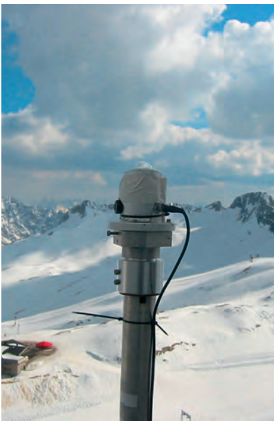
Fig. 4: UVI measurement at UFS with calibrated broadband radiometer. (Koepke)
