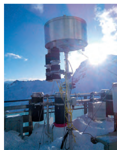
Fig. 5: In the front/top: Filter cartridges for sampling PCDD/Fs which are equipped with heated inlet tubes to avoid freezing (the mouth of the sampling system facing downward). Behind: Funnel adsorber deposition samplers. Picture: GR, LfU
