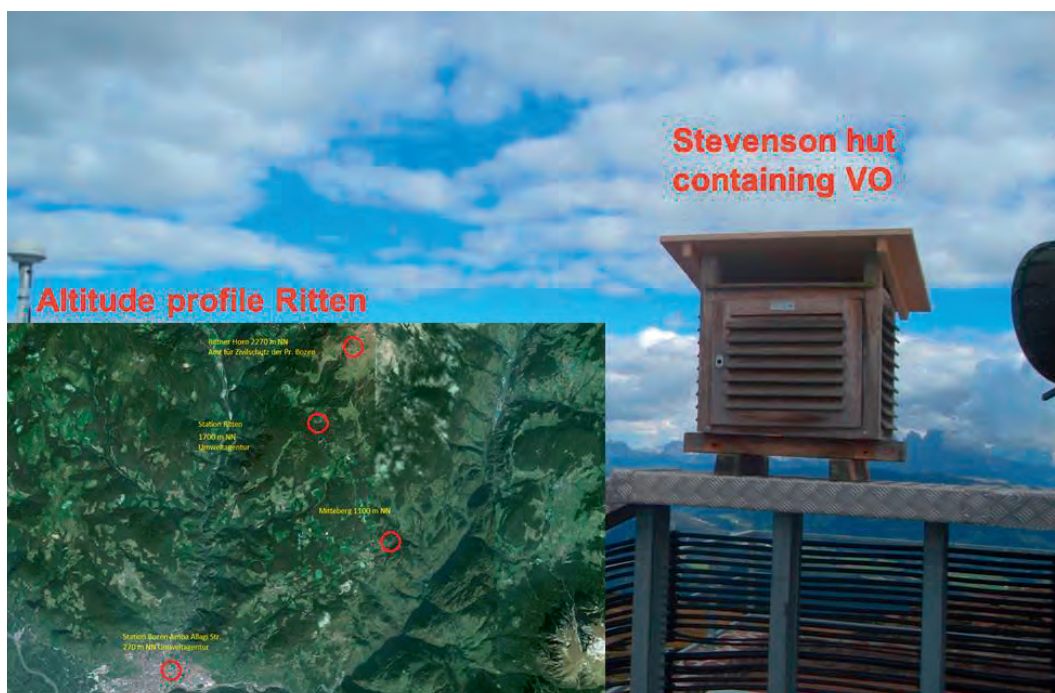
Fig. 7: Picture of Stevenson hut and google map depicting the four locations of the altitude profile which was investigated in the framework of the Virtual Alpine Observatory (VAO)
