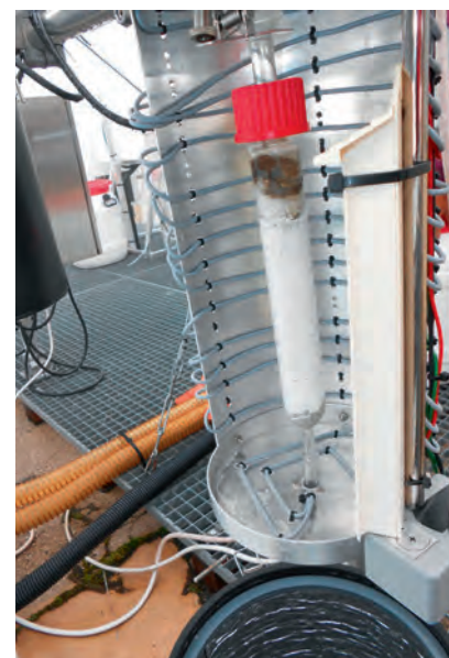
Fig. 7: The interior of the funnel adsorber sampler: in the upper part of the cartridge there is included glass wool in order to collect particulate matter, the white material in the lower part is the adsorbent (XAD-2 resin). Picture: GR, LfU
