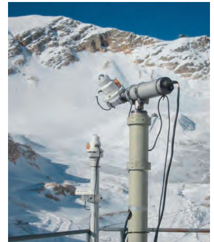
Fig. 5: Measurement of the UVI on tilted surfaces in the skiing area at Zugspitze-glacier with the system ASCARATIS, described in the text. Shown are the moving radiometer, which needs some time to observe all directions, and the radiometer that is permanently in horizontal position to check for unchanged illumination during the observation time. (Oppenrieder et al., 2004)
