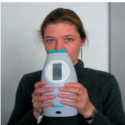
Fig. 5: Measurement of nitrogen oxide (NO) in the exhaled air
