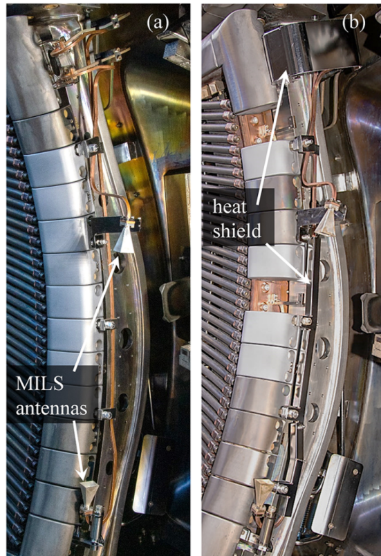
Figure 5: On the left side of the figure the MILS diagnostic is shown as used in the year 2020. From 2021 on, a thermal shield has been installed to reduce expansion of the waveguides, as can be seen on the right side. Figure taken from [12].
