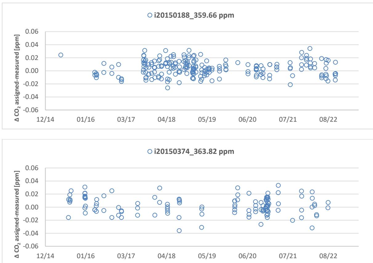
Figure 4: Time series of the offset of CO<sub>2</sub> target measurements to their respective assigned values
