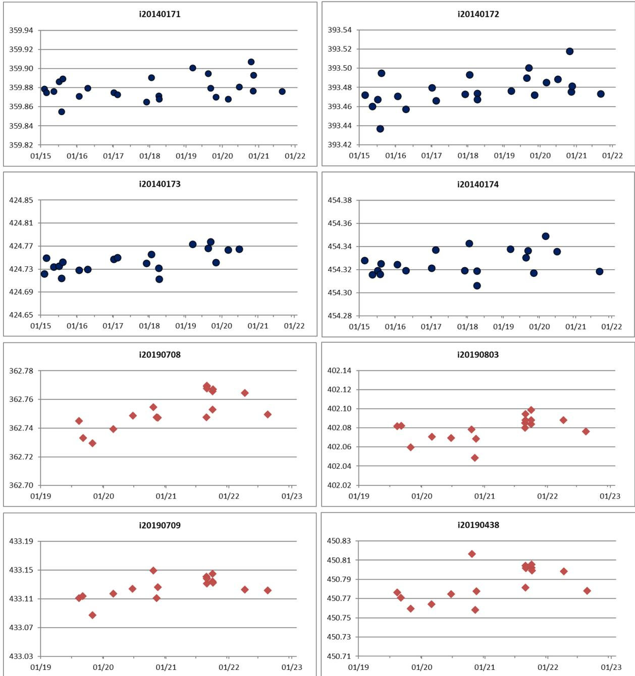
Figure 2: FCL Secondary Standards CO<sub>2</sub> assignment time series (all values in [ppm]).
