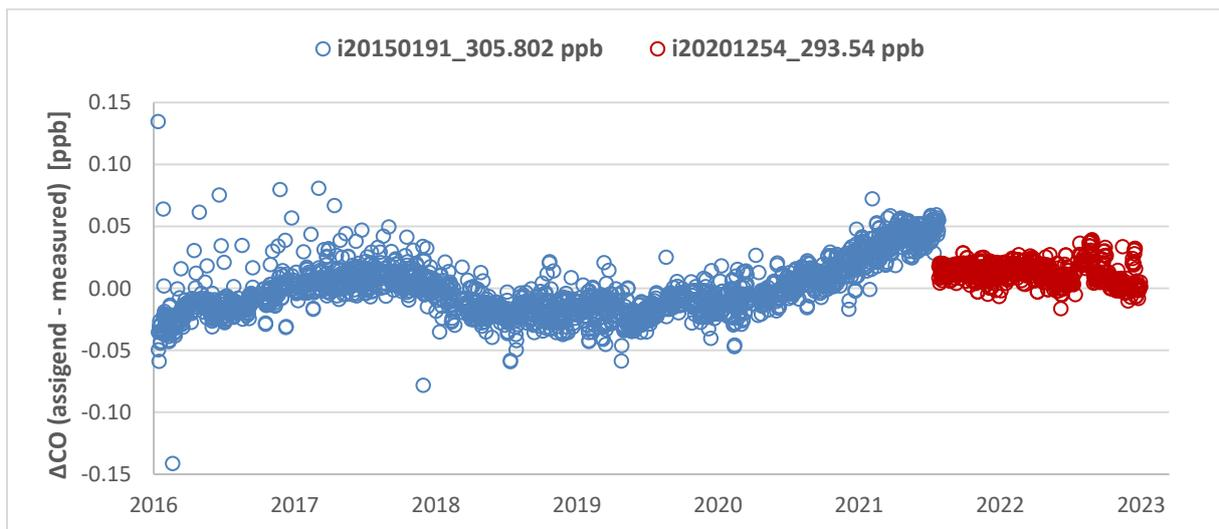
Figure 23: Time series of quadratic regression fit residuals of LGR CO FCL Secondary Standards calibrations
