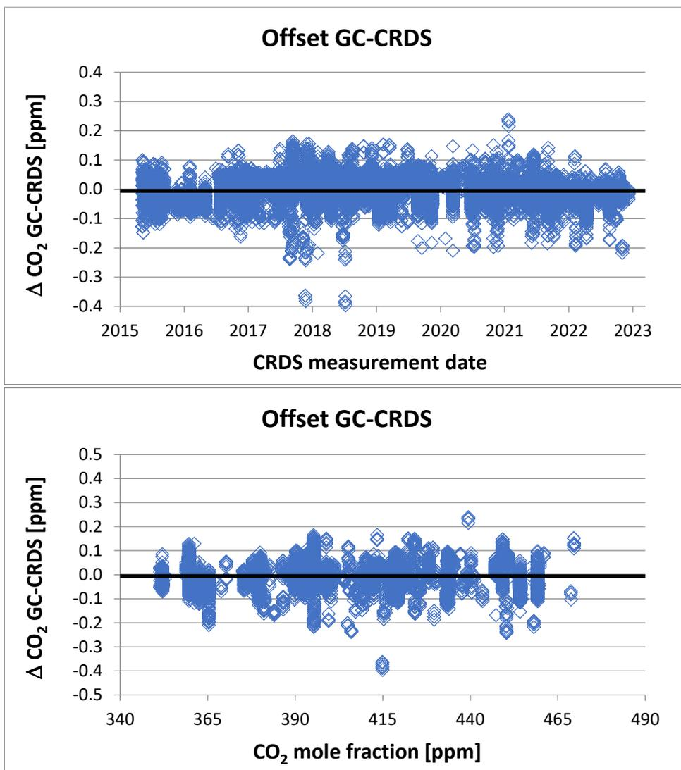
Figure 5: Offsets of daily CRDS CO<sub>2</sub> measurements relative to average GC results. Only analyses results made within one year are considered. The black line represents the mean offset.
