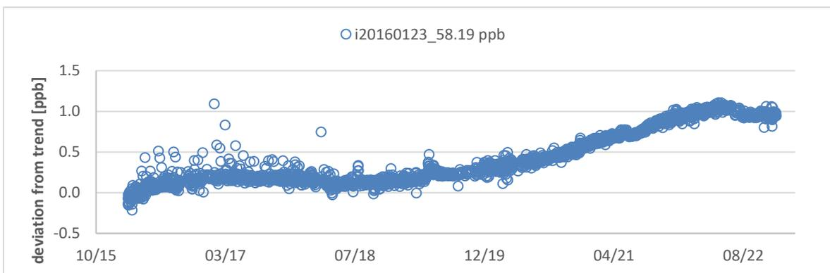
Figure 24: Time series of daily CO residuals data of target standards analyzed on the LGR instrument
