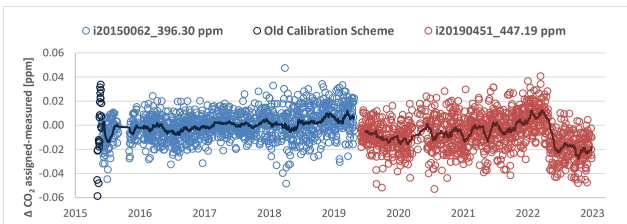
Figure 4: Time series of the offset of CO<sub>2</sub> target measurements to their respective assigned values
