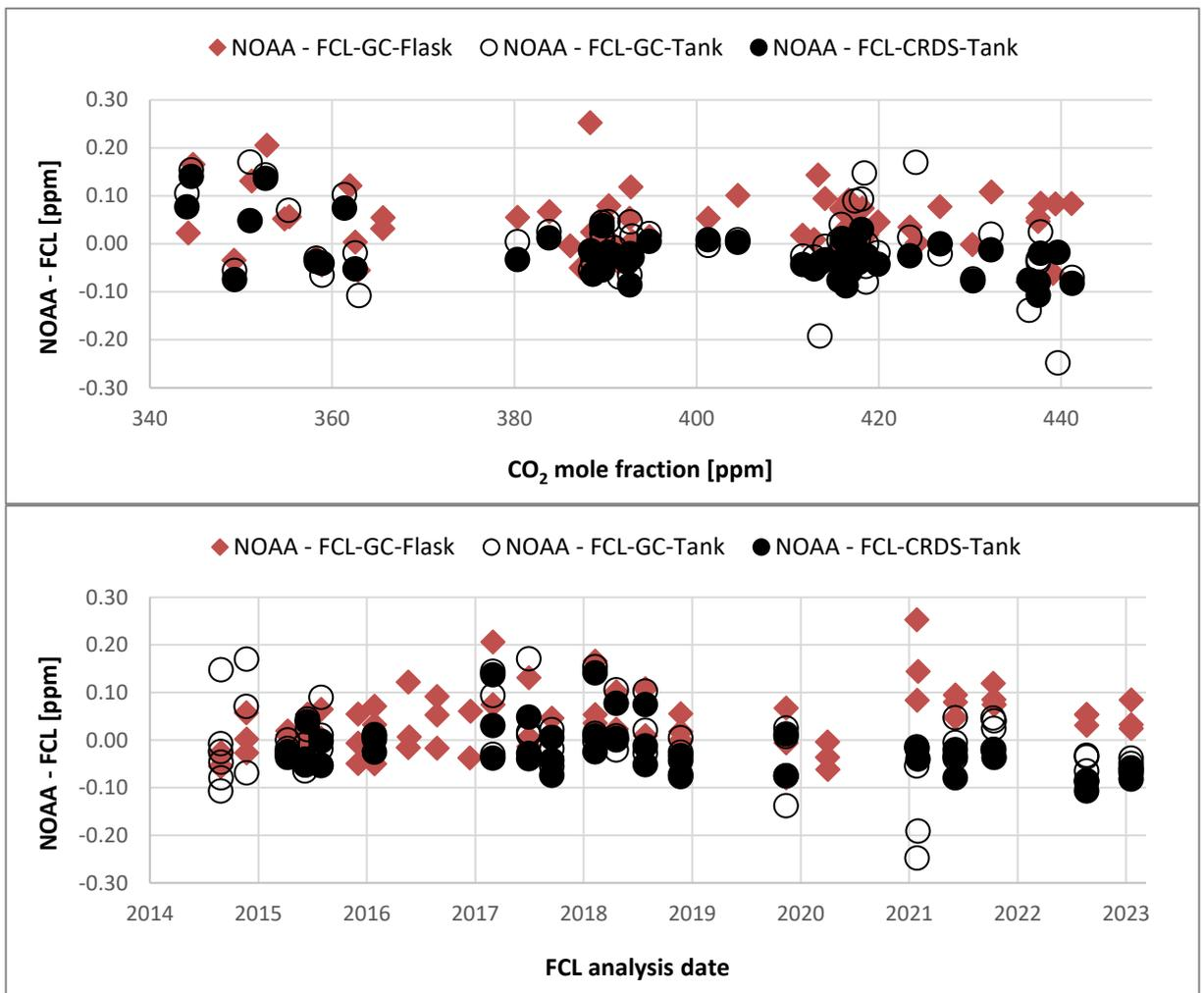
Figure 8: CO<sub>2</sub> offset between FCL and NOAA- based on analyses of flask samples (by NOAA), analyses of flask samples by FCL (GC-FID) and their respective source gases from high pressure cylinders (by FCL using CRDS)
