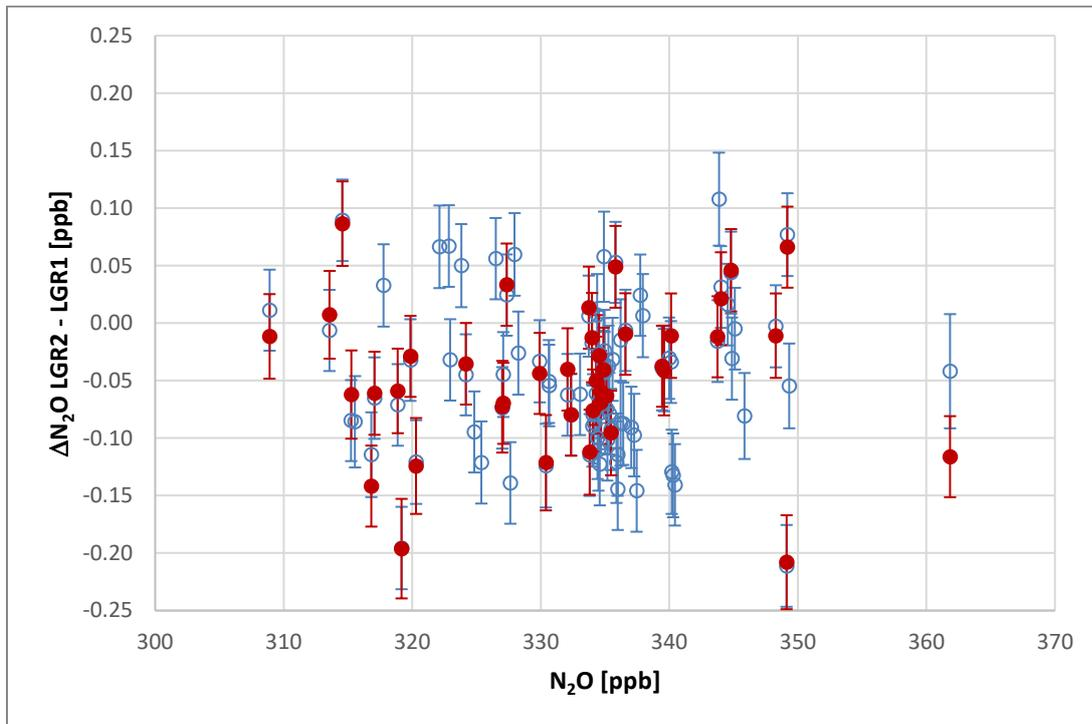
Figure 35: N<sub>2</sub>O offset of two LGR instruments for the same samples
