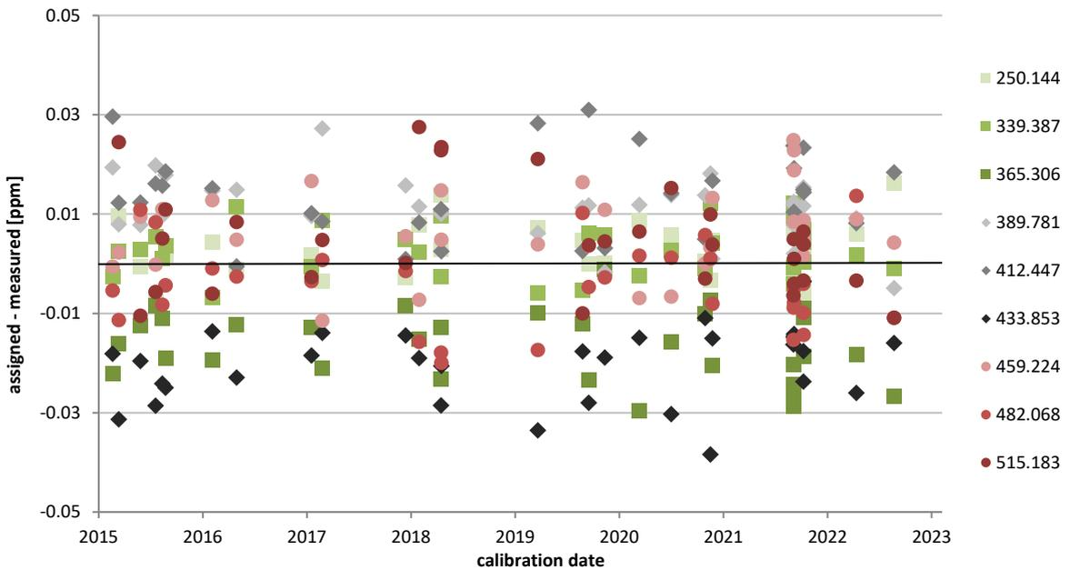
Figure 1: Time series of linear regression fit residuals of the CRDS CO<sub>2</sub> calibration for FCL Primary Standards
