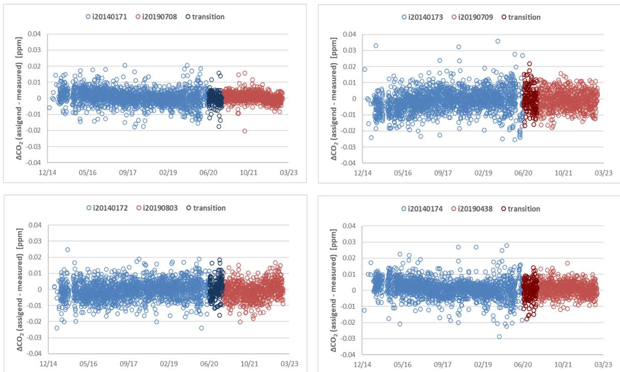
Figure 3: Time series of CO<sub>2</sub> linear regression fit residuals of the FCL Secondary Standards.
