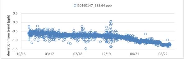
Figure 24: : Time series of daily CO residuals data of target standards analyzed on the LGR instrument
