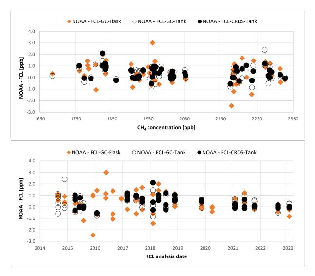
Figure 18: CH4 offset between FCL and NOAA based on analyses of flask samples (by NOAA), analyses of flask samples by FCL (GC-FID) and their respective source gases from high pressure cylinders by FCL (CRDS)
