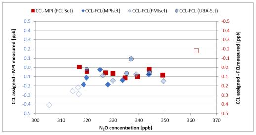
Figure 37: Differences of Primary Standard measured N2O results to CCL assigned values
