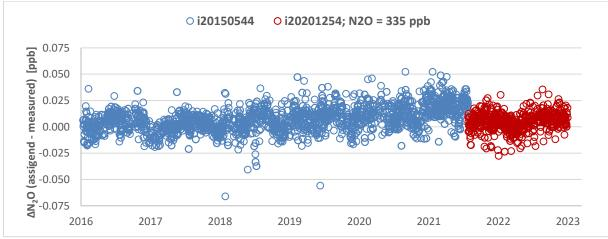
Figure 33: Quadratic regression fit residuals of the daily LGR N2O calibration with FCL Secondary Standards
