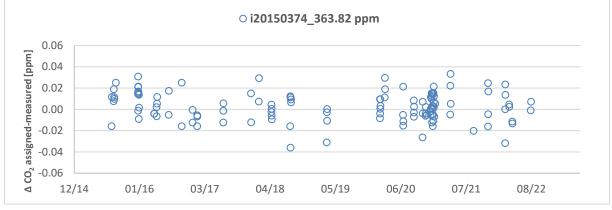
Figure 4: Time series of the offset of CO2 target measurements to their respective assigned values
