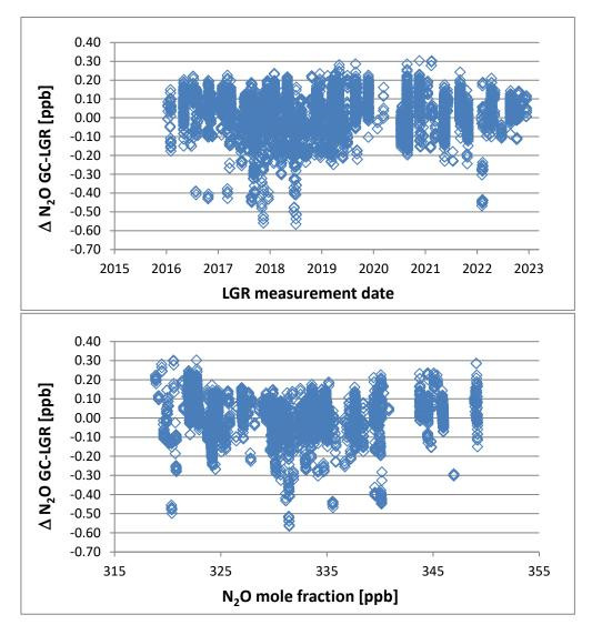
Figure 36: Offsets of daily LGR N2O measurements relative to the annual mean of GC results
