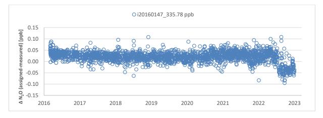
Figure 34: Time series of the offset of the ambient N2O target measurements to its assigned values.
