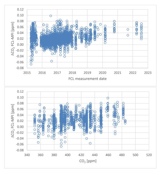
Figure 7: Differences of CO<sub>2</sub> results for samples that have been analyzed at FCL and MPI
