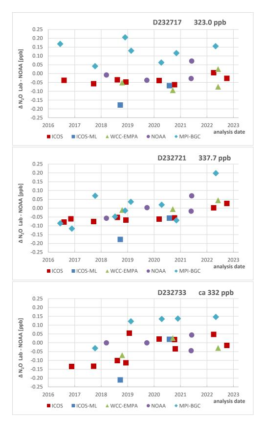
Figure 40: N2O offset in MENI ICP between FCL, MPI, ICOS MobileLab and WCC relative to NOAA
