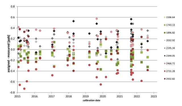
Figure 10: Time series of linear regression fit residuals of CRDS CH4 calibrations for FCL Primary Standards
