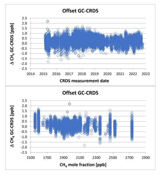
Figure 14: Offset of CRDS daily mean CH4 results relative to GC average results of the same sample.
