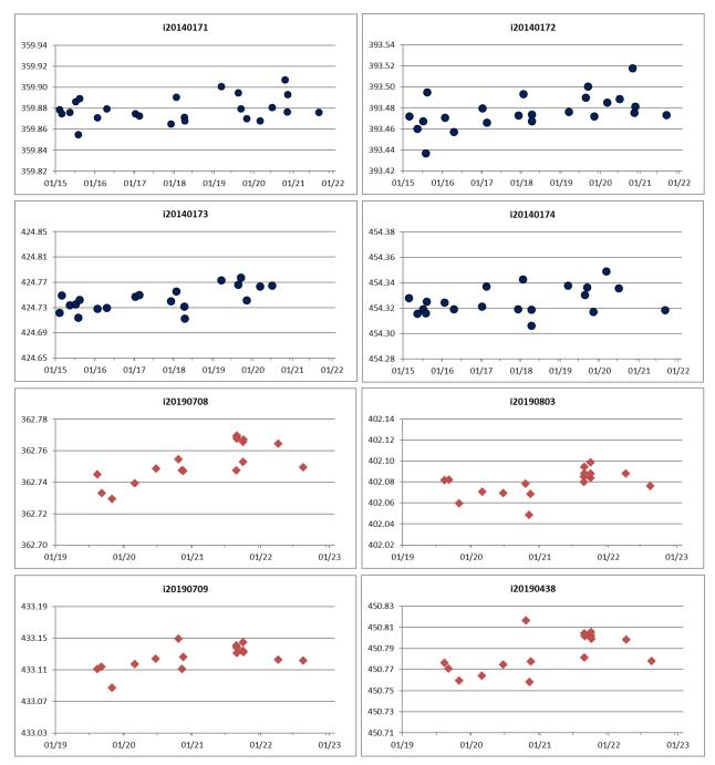
**Figure 2: FCL Secondary Standards CO2 assignment time series (all values in [ppm]).** The dark dots represent the data from the first set, the red diamonds display results of the second set of FCL Secondary Standards.
