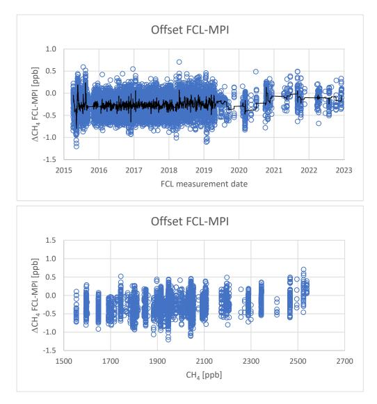
Figure 17: Differences of CH4 results for samples that have been analyzed at FCL and MPI-BGC
