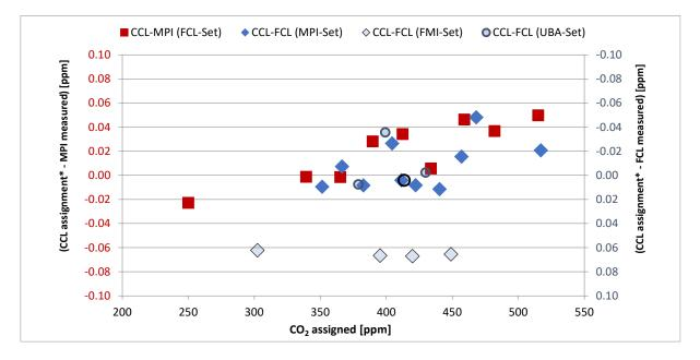
Figure 6: Differences of FCL analysis results of MPI and FMI Primary Standards to CCL CO<sub>2</sub> assignments (blue diamonds) and of MPI-BGC analysis results of the FCL Primary Standards to CCL assignments (red squares).
