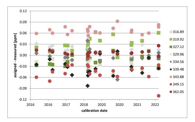
Figure 32: Time series of N2O quadratic regression fit residuals of LGR FCL Primary Standard calibrations
