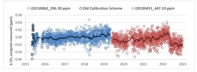
Figure 4: Time series of the offset of CO2 target measurements to their respective assigned values
