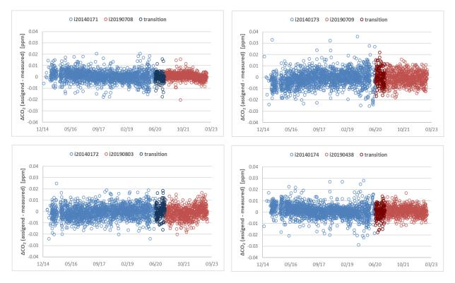
Figure 3: Time series of CO2 linear regression fit residuals of the FCL Secondary Standards.
