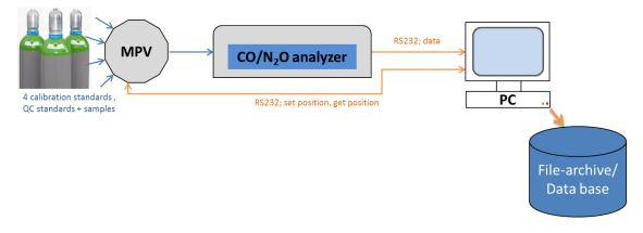
Figure A2.4: Schematics of analysis station, blue lines= sample, orange lines=data/commands
