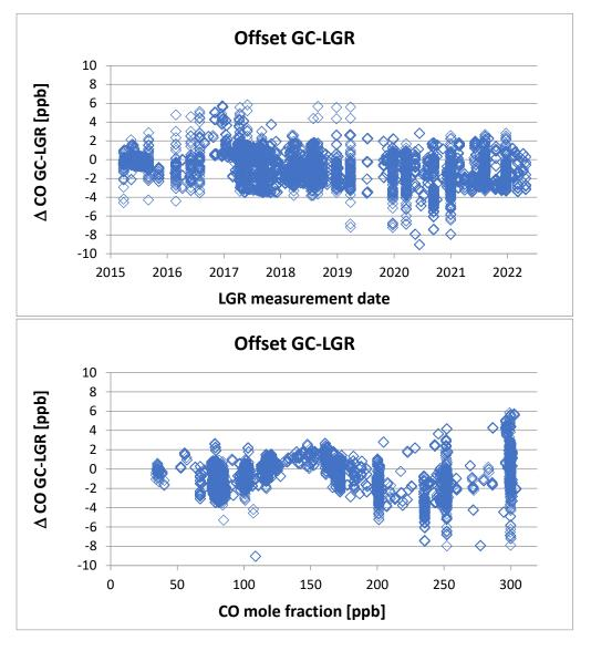
Figure 25: Time series of LGR-GC CO differences of measurement results of the same samples
