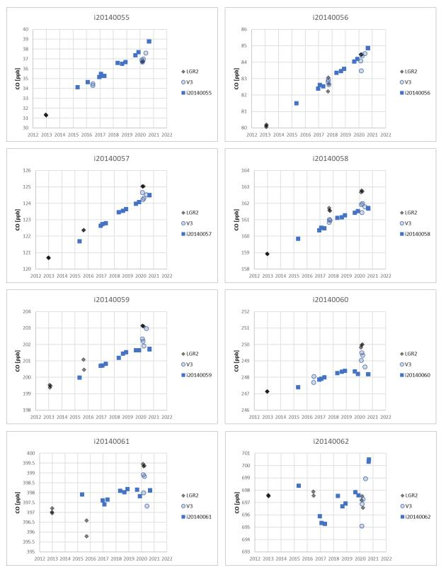
Figure 20: CO Primary Standards, measured at the FCL (blue squares) and at the CCL.
