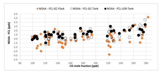
**Figure 29: CO offset between NOAA Sausage flask data and FCL data.** Black dots represent FCL's analysis of the Sausage fill gas (filled symbol: LGR measurement; unfilled symbol: GC); orange diamonds represent GC flask sample analysis
