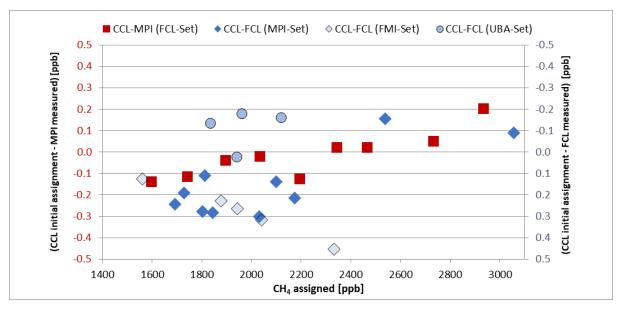
Figure 15: Differences of measured CH4 results to CCL assigned values for FCL Primary CH4 Standards.
