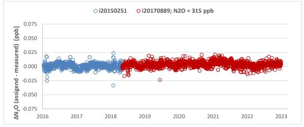
Figure 33: Quadratic regression fit residuals of the daily LGR N2O calibration with FCL Secondary Standards
