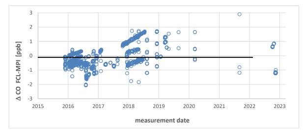
Figure 28: Differences of CO results for samples that have been analyzed at FCL and MPI-BGC
