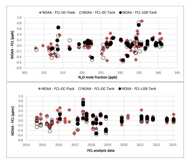
Figure 39: N2O offset between NOAA and FCL based on flask samples
