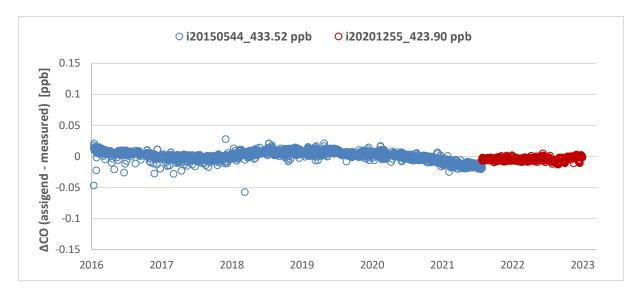
Figure 23: Time series of quadratic regression fit residuals of LGR CO FCL Secondary Standards calibrations
