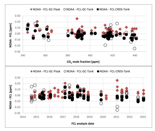
Figure 8: CO2 offset between FCL and NOAA- based on analyses of flask samples (by NOAA), analyses of flask samples by FCL (GC-FID) and their respective source gases from high pressure cylinders (by FCL using CRDS)
