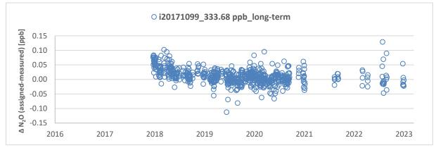
Figure 34: Time series of the offset of the ambient N<sub>2</sub>O target measurements to its assigned values.
