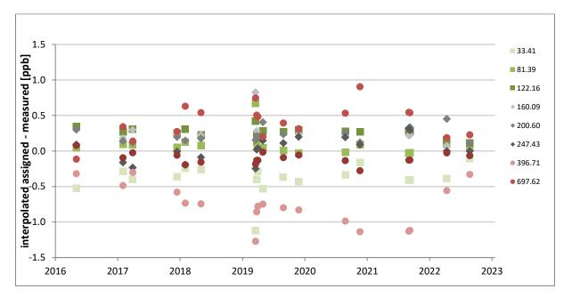
Figure 21: Time series for CO quadratic regression fit residuals of LGR FCL Primary Standard calibrations
