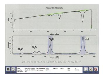
Figure A2.2: Screen shot of spectrum display, upper panel shows photo detector voltage, lower panel shows optical absorption of species of interest.
