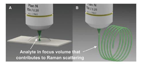
Figure 7: Comparison between the limited collection volume in conventional Raman spectroscopy (A) and the extended interaction volume in FERS (B).
