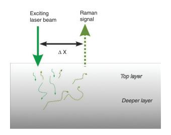
**Figure 11:** Principle of spatially offset Raman spectroscopy. Raman scattered light from deeper layers can be collected in a distance  $\Delta x$  from the spot of illumination. The larger the distance, the higher the ratio of signal from deeper layers, but also the smaller the signal intensity.  $\Delta x = 0$  is equal to the signal collection geometry of conventional Raman spectroscopy.
