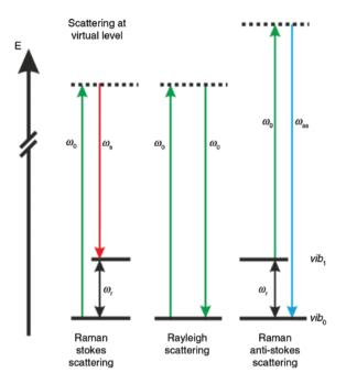
**Figure 2:** Energy level diagram displaying the principle of the Raman effect: incoming monochromatic light with frequency  $\omega_0$  is scattered either elastically (Rayleigh;  $\omega_0$ ) or inelastically with energy transfer to (Raman Stokes scattering;  $\omega_s$ ) or from (Raman anti-Stokes scattering;  $\omega_a$ ) the molecule.
